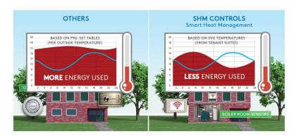
Other controller systems rely solely on a single sensor outside the building, so are only able to loosley follow the daily temperature changes, providing merely a gross approximation to the actual heating required.
