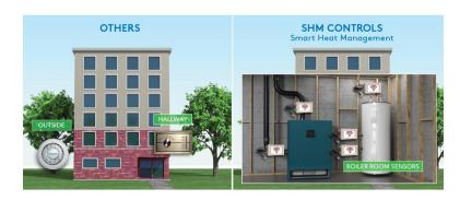
In comparison, a building equipped with the SHM Controller, would have a wireless temperature sensor outside the building, but that is just the beginning. In order to have accurate readings of any situation and be able to predict heating requirements, the SHM Controller has several wireless temperature sensors strategically placed inside the boiler room on pipes, boilers and hot water tanks.
